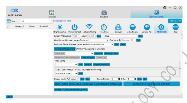
3. Click Use LedSet4.0 to configure the LED module at the bottom of the Advanced Settings screen to open the LedSet4.0 software interface.
