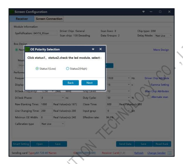
10. Click "Next Step" to enter the "scan line number" window and select the scan line according to the actual display of the current module.
