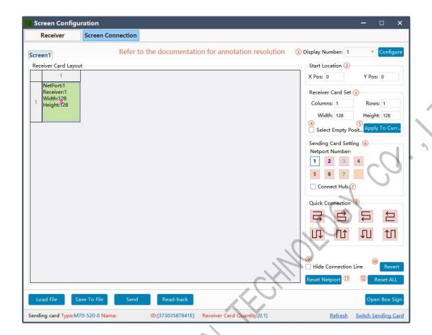
23. Click send and choose "as the main sender" and save to device; or choose "As the backup sender" to save to backup sender device. For double sender backup only work for synchronous controller.
