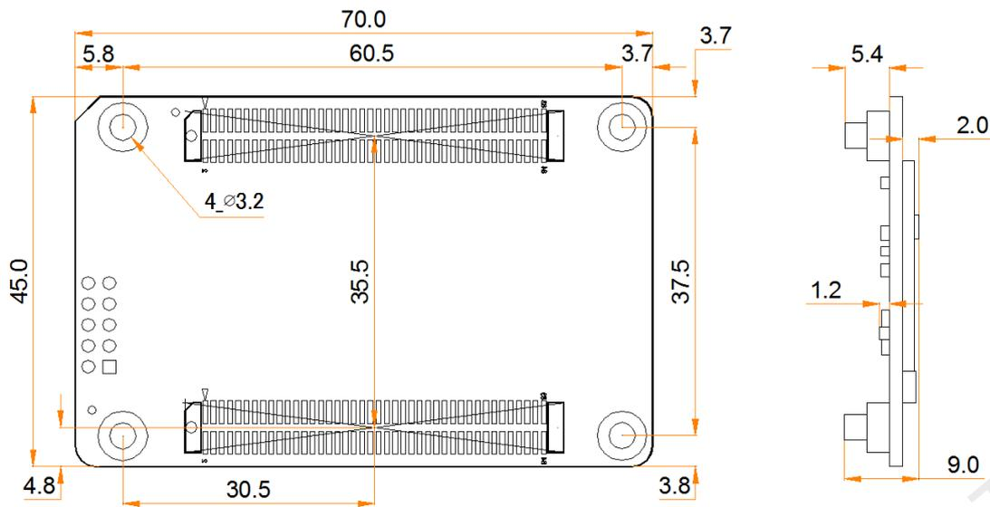
Tolerance: ±0.1 Unit: mm
