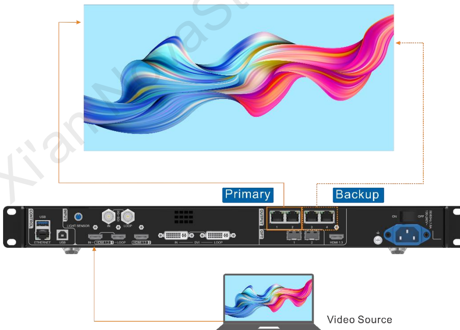
Figure 5-27 Ethernet port backup connection
