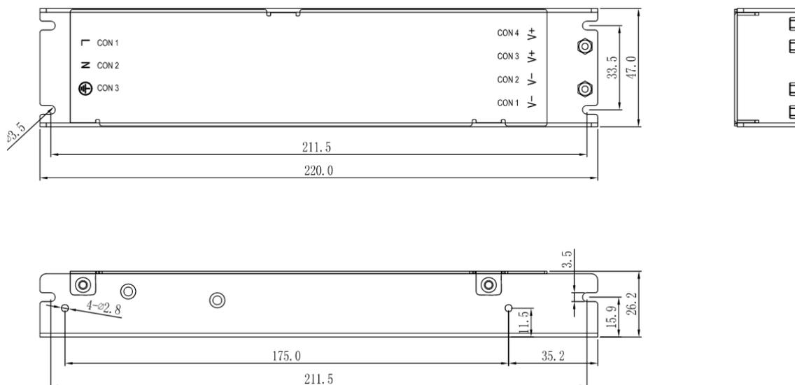
8.3. Pin connection. 连接器脚位定义:
