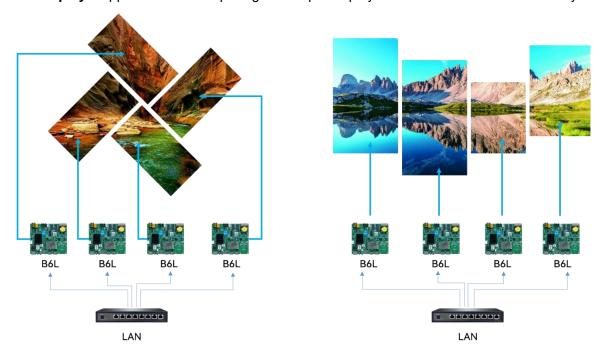
4. **Multi-screen synchronization display**: Multiple independent displays synchronously display the same image at the same time.
