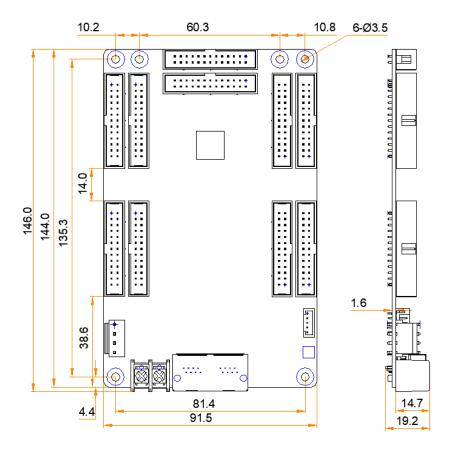
Tolerance: ±0.3 Unit: mm
