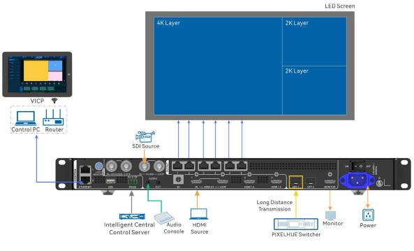
Ethernet Cable Video Cable Audio Cable Control Cable Optical Fiber Cable
