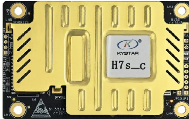
Figure 1 Front view of the H7s-c receiving card
