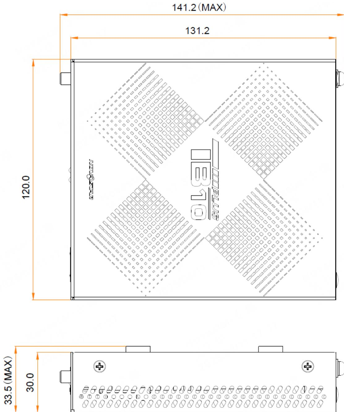
Tolerance:  $\pm 0.3$  Unit: mm
